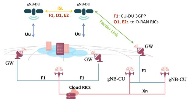
Fig. 3. High-level system architecture.
